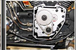
giving it another careful inspection to ensure that there is adequate clearance for all moving parts within the cam chest.
