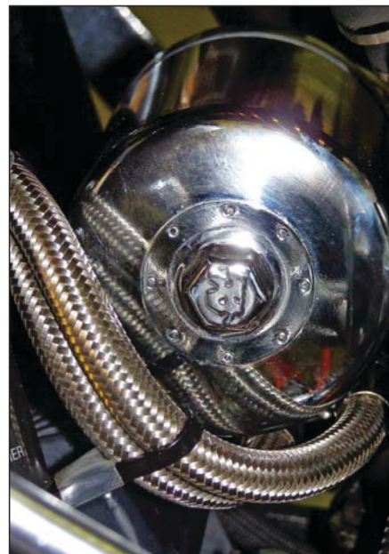
The K&N filter mounts in the original filter's location, and the two braided lines are routed down to the filter cooler. Note the two zip ties that prevent the braided lines from rubbing against the frame.
