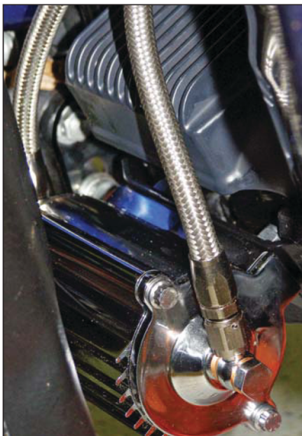
The Feuling Oil Filter Cooler hangs down in front of the engine where it receives its fair share of fresh, cool air. As you might guess, this helps dissipate heat from the oil circulating through the filter.
